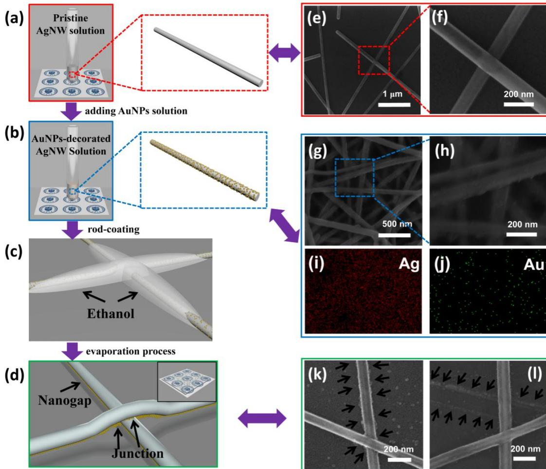
Figure 1: Schematic of fabrication procedures and corresponding SEM images of AgNW film. (a,b,c,d) Schematic of fabrication procedures, the insert of (d) is the schematic of entire AgNW film. SEM image of (e,f) pristine AgNW film, (g,h) AuNPs-decorated AgNWs. (i,j) EDX mapping of (g). (k) SEM image of self-assembled AuNPs on AgNW film and (l) the trace of self-assembled AuNPs.
